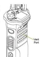
Your radio is designed to be submerged to a maximum depth of 6 feet, with a maximum submersion time of 2 hours. Exceeding either maximum limit may result in damage to the radio.
