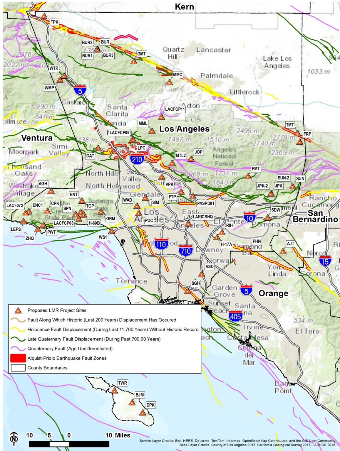
Figure 3.5-1: Mapped Faults within Proposed Project Area
