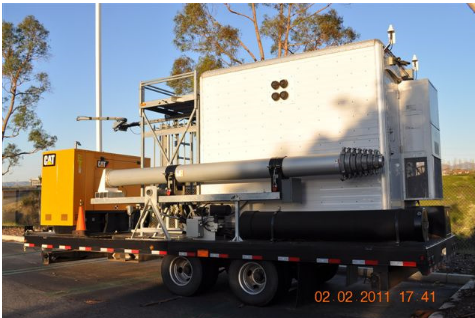
Figure 8: Example of Typical Small Mobile Cell On Wheels Equipment Ready for Transport (COW Sites)
