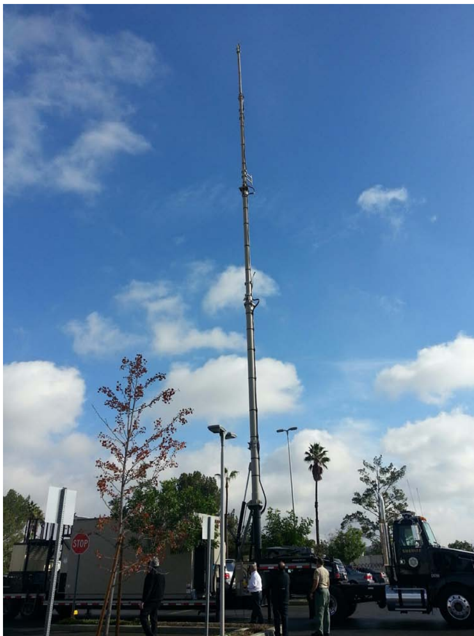
Figure 9: Example of Typical Large Mobile Cell On Wheels Equipment Deployment (COW Sites)
